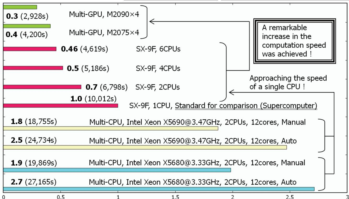
Bold numbers indicate the speed ratio with respect to a single CPU on the SX-9F (NEC supercomputer).
